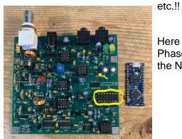
Here is the 20m Phaser alongside the Nano Every. Only four wires will extend from the Nano to a 14pin DIP header that will replace the PIC processor on the Phaser board (yellow oval).
