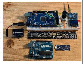
The control knob selects the operating frequency to be sent to the si5351 breakout board (upper right), The OLED display shows the current frequency and step size. Surprisingly, this layout was just published as part of an article in this months QST. Great Minds,
